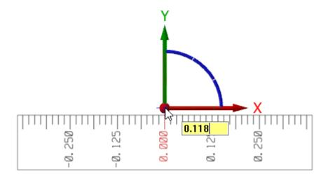
21. Press [Enter] a second time to verify the move, and then, in the **Dynamic** function panel, click **OK and Create New Operation**.
