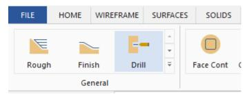
2. In the Lathe Drill dialog box, select the T1111 tool.
