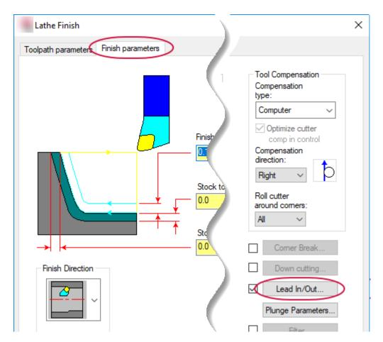
7. Select the **Lead out** tab, set **Angle** to **-90.0** and **Length** to **0.02** as shown in the following picture.
