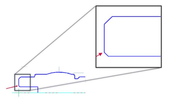
8. If necessary, change Feed rate to 0.002, Spindle speed to 2000, and Max spindle speed to 5000.
