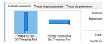
3. On the **Thread shape parameters** tab, set the parameters as shown in the following image. You can also use the **Select from table** button to choose the parameters that are appropriate for the threading operation.
