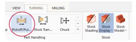
3. In the dialog box, choose **Pickoff, cutoff**. Note that **Pickoff, cutoff** is the only part-handling operation shown in the dialog box that is used with Swiss.
