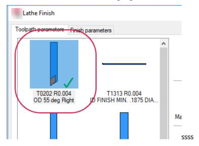
4. Set Feed rate to 0.002, in/rev and Spindle speed to 2000, RPM, as shown in the following picture.
