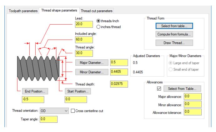
4. On the **Thread cut parameters** tab, select **Box** in the **NC code format** drop-down. **Box** is a G92, **Canned** is G76, and **Longhand** is G32.
