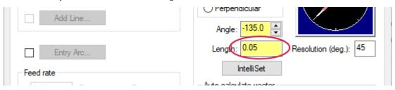
12. On the **Second pass Lead in** tab, set the direction indicator so that it is pointing straight down (-90 degrees), change **Length** to **0.05**, and click **OK**.
