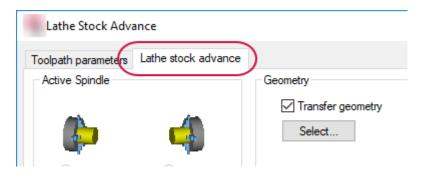
5. Deselect **Transfer geometry**. This prevents the stock from repositioning as would happen with a stock pull on a lathe.
