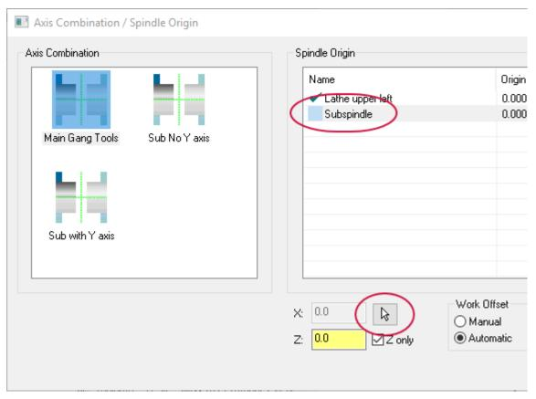
7. Select the 0 point of the part on the subspindle, as shown in the following picture, and click **OK** in the **Axis Combination / Spindle Origin** dialog box.
