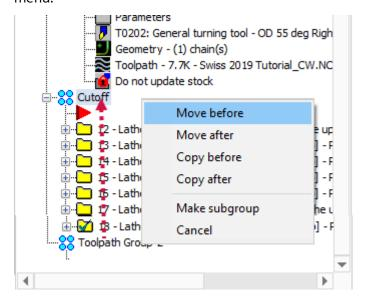
On a Swiss machine, the cutoff must be the last operation, and the order of the toolpaths in Toolpaths Manager must reflect this requirement. However, you could not create this operation before you had created the cutoff, which is why the new toolpath group must be moved now.
