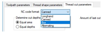
5. Set **Number of spring cuts** to **1**, **Number of cuts** to **8**, **Acceleration clearance** to **0.1**, and then click **OK**. You should see the threading toolpath shown in the second picture following.
