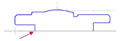
6. Use Backplot to test the toolpath.
