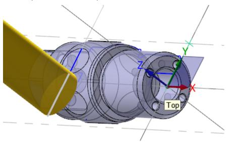
12. On the **Lathe Milling** contextual tab, select **Toolpath Transform**.
