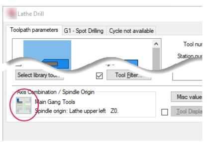
4. The machine you are using for this tutorial has no Y axis, so ensure that the **Sub No Y Axis** axis combination is selected.
