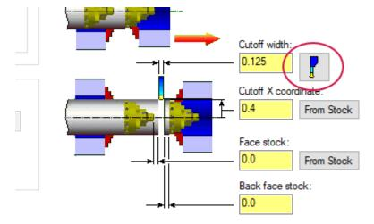
9. The cutoff X coordinate of 0.4 is derived as follows: The stock's diameter is 0.75. The 0.4 is a radius, so it represents a diameter of 0.8, which gives you 0.5 per side above the stock.
