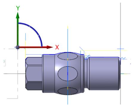
26. Regenerate operations 11 through 17, and backplot the **Cutoff** group operations to see the cutoff in action.
