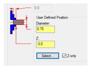
**Z** is the distance between the tool and the face of the chuck jaw or guide bushing and must be entered as a negative number. Typically, you subtract about **0.5** inches from the full **Z** value. This extra space leaves room for the cut-off tool to perform its operation. Failure to set this value properly can lead to collisions during machining.
