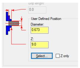
The **Z** here is the distance between the main spindle and the subspindle.
