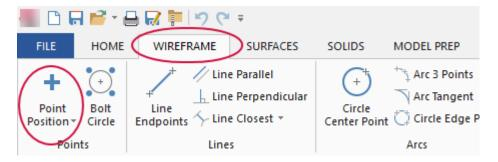
10. Create a point similar to the one shown in the following picture (in other words, your choice need not exactly match the one shown), and click **OK** in the **Point Position** function panel. Note that the point you select must be above the centerline of the part and beyond the face of the part.
