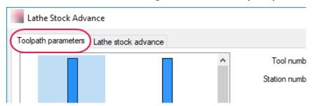
3. Select tool number **T450142**, the stock advance dummy tool. The operation requires that a tool be selected, even though it will not use it. Selecting a tool that will not be used with Swiss Lathe eliminates later conflicts in Mastercam.
