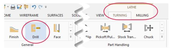
2. In the **Lathe Drill** dialog box, choose tool **T2121 0.1875**. Several tools start with T2121, so be sure you pick the correct one.
