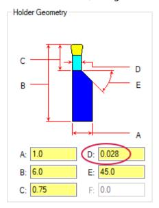
8. Back in the **Toolpath parameters** tab, set the parameters as follows:
