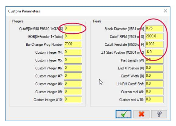
These values are used in the NC code's header section and are the values needed when you select 1 for **Cutoff**, the first integer in the list. By choosing 1, you specify that the machine is equipped to handle G266.
