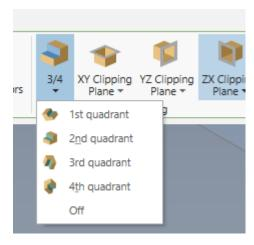
Part sectioning displays your stock in 3/4 sections using a combination of two clipping planes. Once you select a section, you can click and drag either plane to adjust the view.
