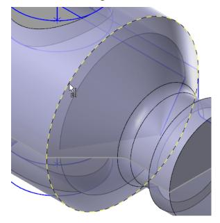
A built-in calculator reads the dimensions of the selected arc directly into the Rotary diameter field.
