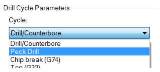
The name that appears on this tab depends on the cycle you select in the **Drill Cycle Parameters** drop-down list. The cycles which are available to you depend on the active control definition.
