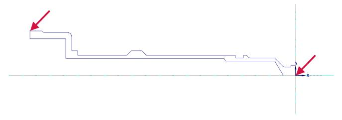
Mastercam calculates the distance between the points and enters the values of the part's outer diameter (OD) and length directly into the fields.
