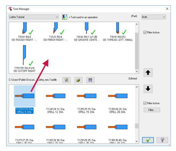
When you create or work on a tool in the part window, you are working on a tool definition that is stored in the machine group. That means if you edit a tool from the part window, you are only changing the definition in the machine group and not the tool library. If you import the tool from another Mastercam file, the changes you make here will not appear in the original file.
