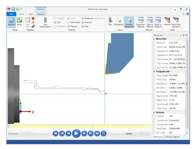
4. Select the Initial Stock option in the ribbon bar's Visibility group to see the stock before machining.
