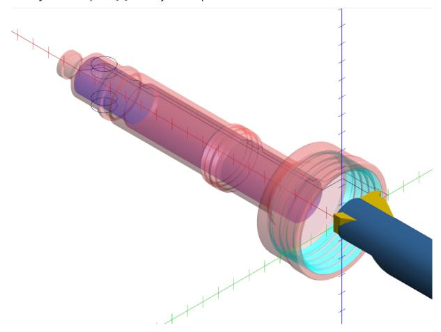
Although you are able to view the operations through the translucent stock, Mastercam Simulator's clipping plane and part sectioning tools offer an even better view of the part's interior.
