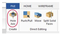
b. [Ctrl + click] the internal face of the upper hole to select both openings of the through hole.Use [Ctrl + click] to select faces with matching diameters.
