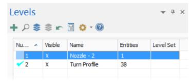
2. Create a Level 3. Name this level, C-Axis Geometry.
