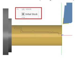
6. For a better view of the operations in the Mastercam Simulator, use the **Page Up** key to zoom into the part and [**Ctrl + Arrows**] to pan the view.
