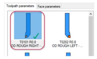
Mastercam uses different colors to represent the orientation of lathe tool inserts.
