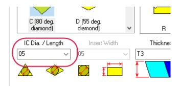
This value defines the insert's IC diameter or length (depending on the selected shape). The IC diameter (IC = inscribed circle) is determined by placing a circle in the insert shape and measuring the circle's diameter.
