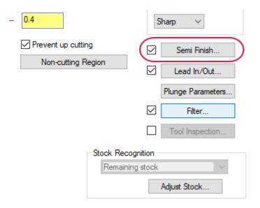
The arc motion of the dynamic toolpath can leave an uneven surface. After the rough passes, the semi-finish pass follows the contour of the part with the roughing tool, smoothing and preparing it for the finish operation.
