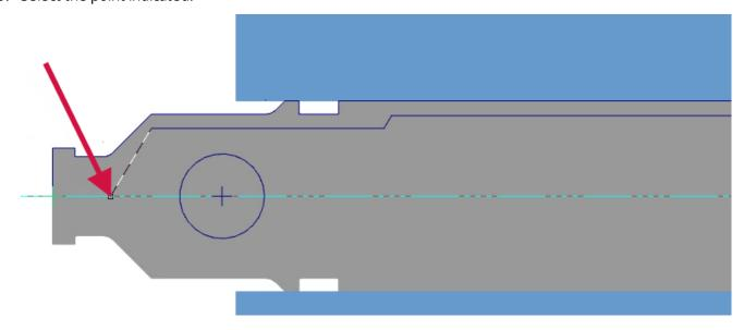
Mastercam returns you to the **Lathe Drill** dialog box and automatically enters the correct value in the **Depth** field.
