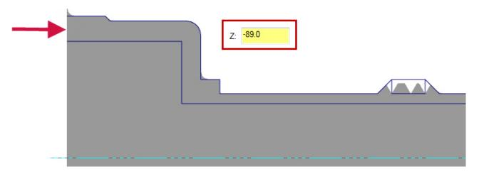
As indicated by the image in the dialog box, the point you select (Z -89.0) will be transferred to Z0 after the stock flip operation
