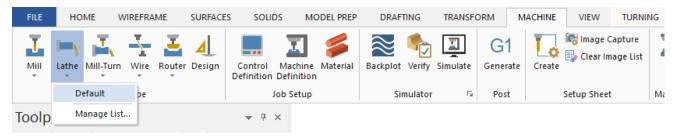
The menu lists all available machine definitions. This tutorial uses Mastercam's default Lathe machine. Normally, you would select the machine on which you plan to cut the part from the list displayed here.
