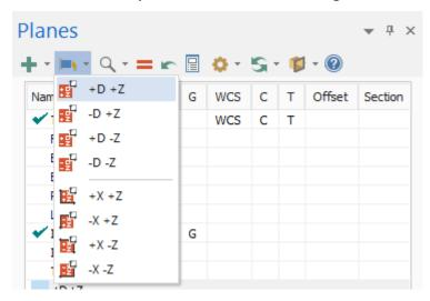
When working with a lathe, you can orient the construction plane to work in radius (X/Z) or diameter (D/Z) coordinates.
